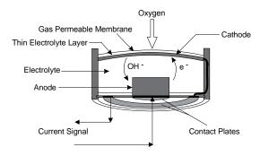
Fig. 3.9 Trace Oxygen sensor design principle
